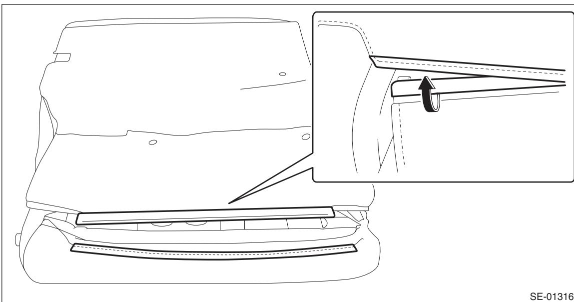
6) Remove the plastic hooks on the back side of the backrest assembly LH.
