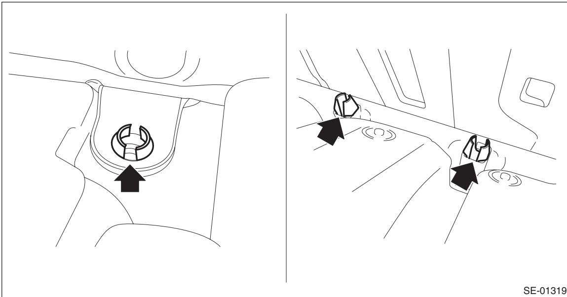
9) Remove the pad assembly - main LH from the frame assembly - rear backrest LH.
