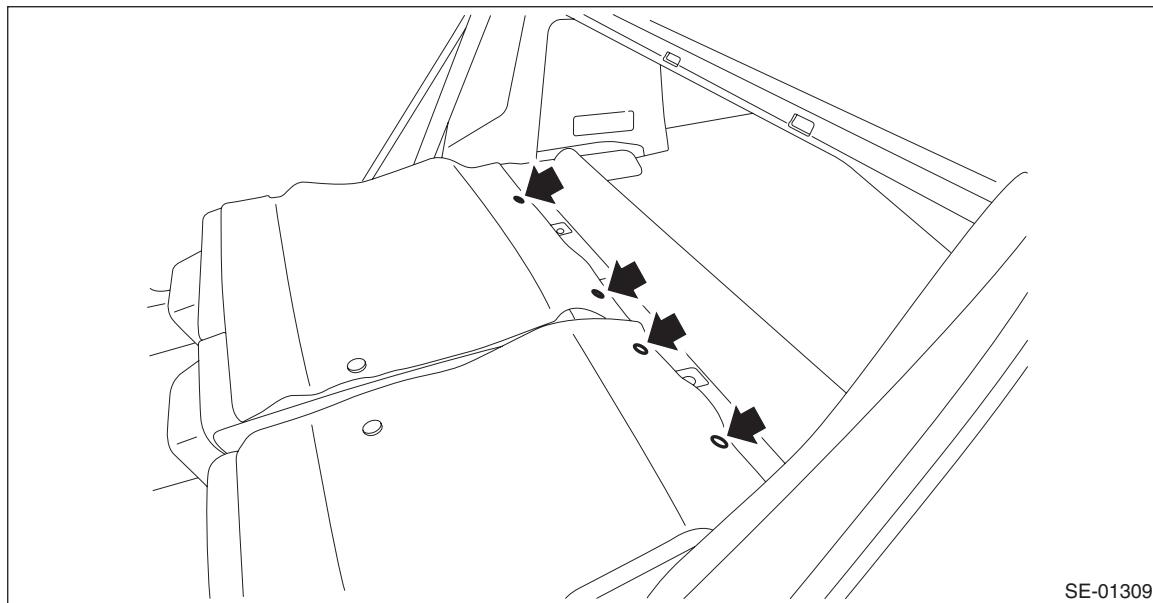
(3) Turn over the cover COMPL - rear backrest LH to remove the bolts.
