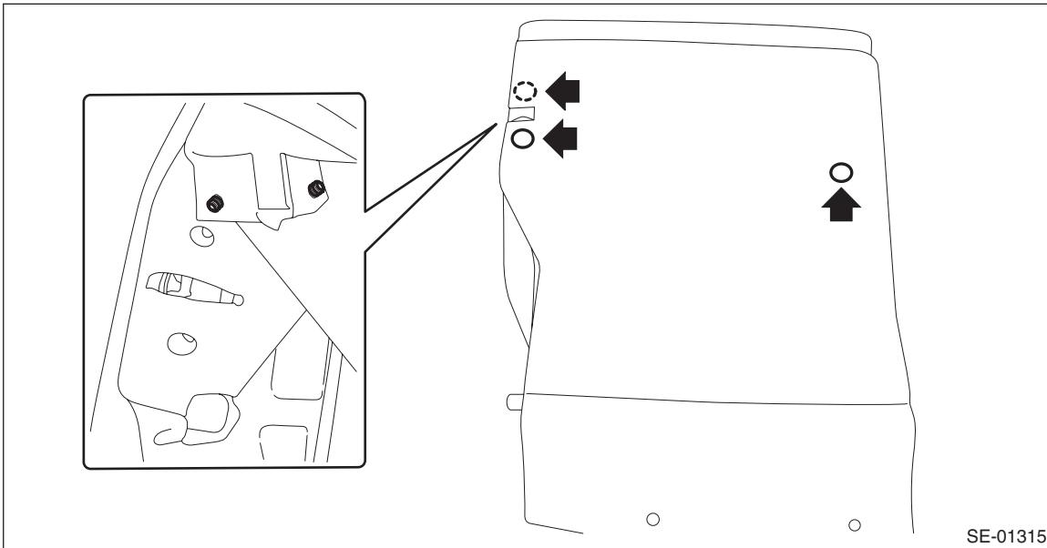
5) Detach the plastic fastener at the bottom of backrest assembly LH and turn over the cover COMPL - rear backrest LH.
