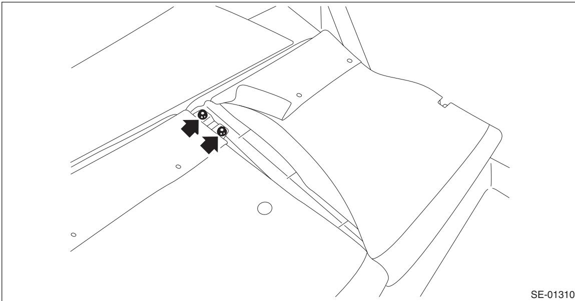
(4) Remove the backrest assembly LH from the hinge assembly.
